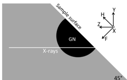
**Figure 1.** Sketch showing a side view of the X-ray scanning position relative to the selected graphite nodule (GN, shown in black). The white line represents the projection of the mapping plane illuminated by the incoming X-rays, which are along the Z direction. The laboratory coordinate system (X, Y, Z) and sample coordinate system (X, H, F) are defined.
