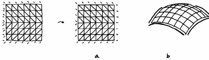
Figure 9. Vertical supported translation faceted elliptic paraboloid. a) The translation truss system. b) The faceted translation shell.
