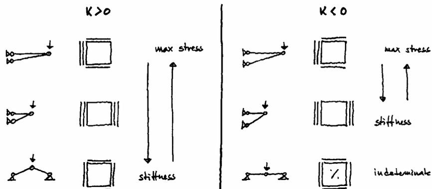
Figure 10. The stiffness of the previous examples illustrated by plane truss analogies.
