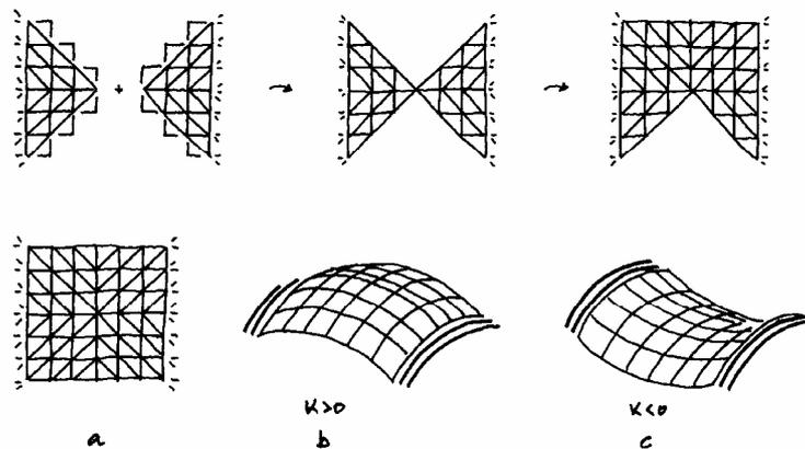
Figure 8. a) The construction of the translation truss system from 4 successively built systems. b) Facetted translation shell with positive Gaussian curvature. c) Shell with negative Gaussian curvature.
