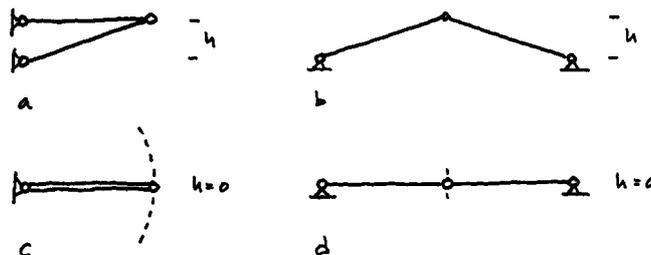
Figure 2. Plane systems illustrating the definitions below. a) and b) Statically, kinematically and geometrically determinate systems. c) Statically, kinematically and geometrically indeterminate system. d) Statically and kinematically indeterminate but geometrically determinate system.
