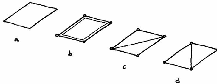
Figure 4. a) A quadrangular facet. b) Structural system consisting of bars and a plate. c) and d) Equivalent structural systems consisting of bars.
