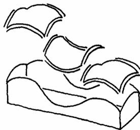
Figure 15. Configuration illustrating the support conditions for the three sections. One line along the edge of a shell indicate that the edge is single supported.
