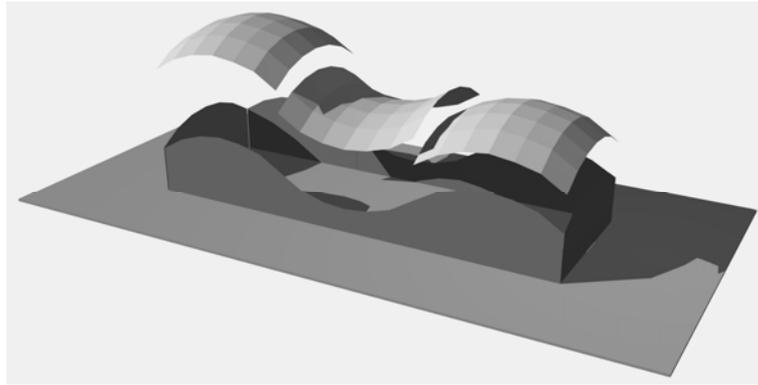
Figure 14. The considered structure is covered with one translation shell composed of three sections having respectively positive, negative and positive Gaussian curvature.
