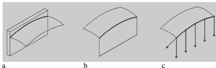
Figure 6. Examples of supports. a) Double support. b) and c) Single supports.
