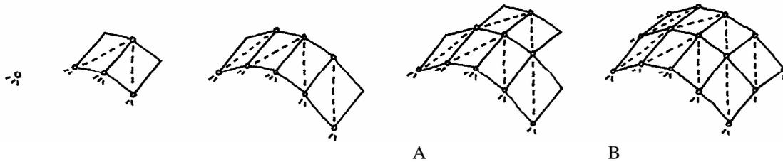
Figure 5. Successively built translation truss systems. A: System that is supported in two directions at every joint along one edge. B: System that is supported in two directions at every joint along one edge and in one direction at every joint along the two edges on each side of this.
