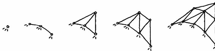
Figure 3. The principle of successively built spatial truss systems. The first joint is supported in three directions, the second joint is secured by one bar and supported in two directions. The rest of the system is built by subsequently adding joints, so that each joint is kinematically and statically determined by either one bar and two supports, two bars and one support or three bars. A support is illustrated by a short line.
