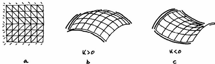
Figure 7. a) The successively built translation truss system. b) Facetted translation shell with positive Gaussian curvature. c) Shell with negative Gaussian curvature. Two lines along an edge indicate that it is double supported, one line along an edge indicate that it is single supported.
