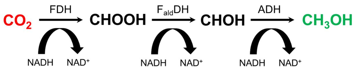
Fig.1 Biocatalytic transformation pathway of CO<sub>2</sub> to CH<sub>3</sub>OH via stepwise reverse enzymatic catalysis by FDH, F<sub>ald</sub>DH and ADH as first introduced by Obert and Dave [7].
