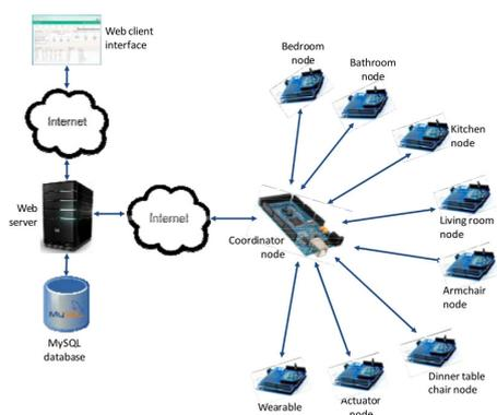
Figure 1: Architecture of the considered environmental sensor network (picture taken from (Dasios et al., 2015)).
