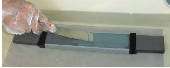
(a) Application of epoxy on steel
