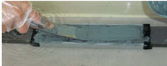
(c) Surface sealing layer of epoxy
