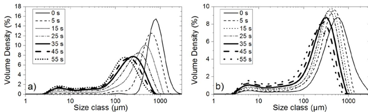
**Figure 2.** Particle size distributions of *A. nidulans* A4 samples taken from the high shear mixer at short time intervals, i.e. 0 s, 5 s, 15 s, 25 s, 35 s, 45 s and 55 s. a) PSD from a broth sample removed from the shake flasks after 15 h growth. b) PSD from a broth sample removed from the shake flask after 52 h growth.
