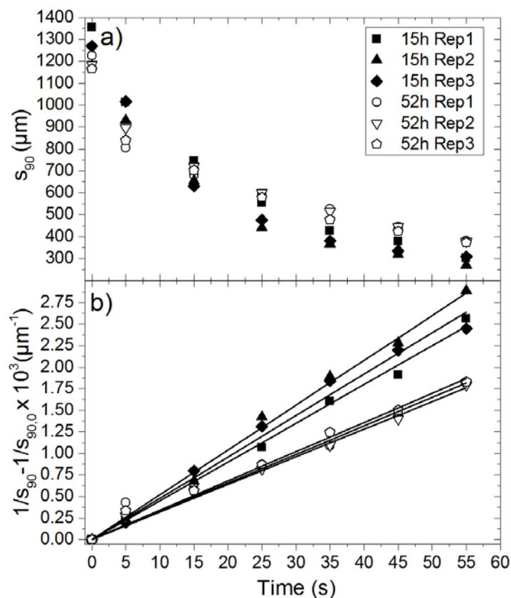
**Figure 3.** Preliminary results from the fragmentations test performed in *A. nidulans* A4 grown in complex media, samples taken at different fermentations times: 15 h (■, ▲, ◆) and 52 h (○, ▽, ◇). a) Evolution of the 90<sup>th</sup> percentile of the PSD in the high shear mixer. b) Results after the normalization with Equation. (1). the slope of the curves corresponds to the relative fragmentation rate,  $k_{\text{frag}}$ .
