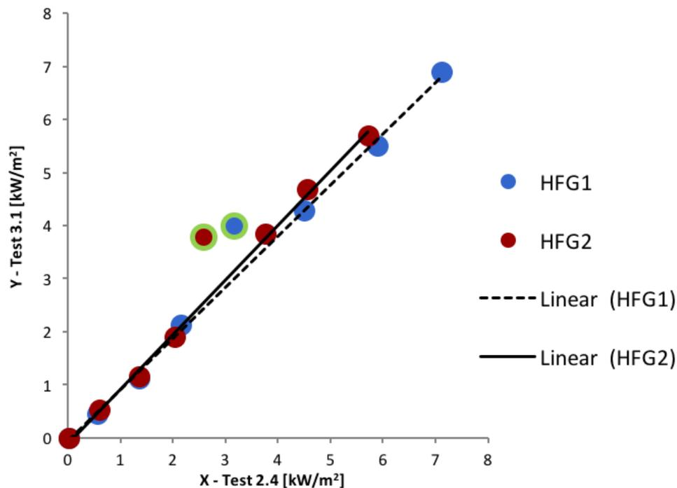
Figure 10. Two-dimensional scatter diagram of the paired data set from test 2.4 and 3.1, with and without the paired data for a HRR of 4 kW. The two green lines encircle the two measurements made with a HRR of 4 kW and the two linear trend lines ignores these two measurements.
