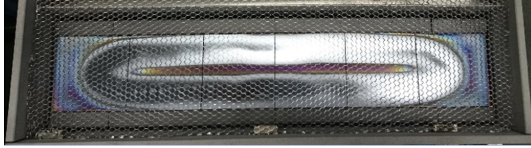
Figure 4: Image of an SSM accommodating target material divided into several tiles. A honey comb collimation grid is placed 50 mm from the target surface. © VON ARDENNE Corporate Archive
