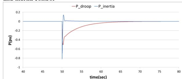
Fig.9 Individual power commands produced by the two independent classic controllers-Scenario A
