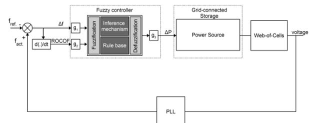
Fig. 3 Implementation of the proposed control for combined frequency containment and inertial response
