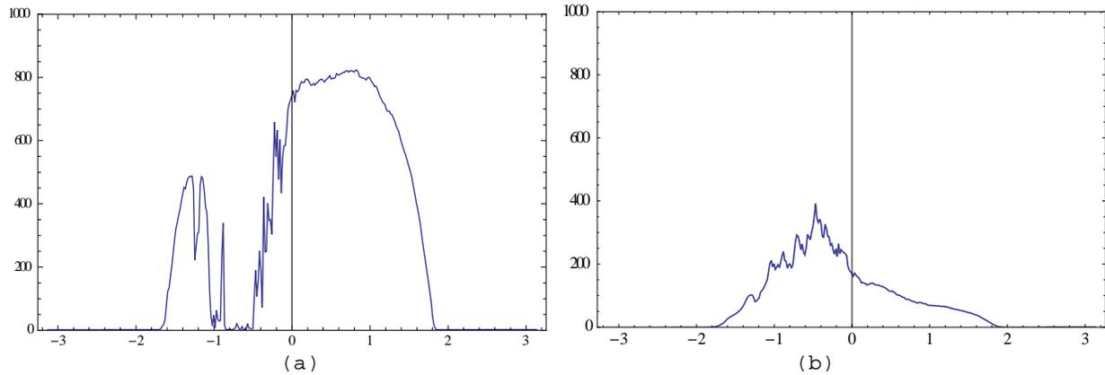
**FIGURE 5.** Solar data obtained near Copenhagen at the 10<sup>th</sup> April 2017 are plotted as a function of azimuth angle (rad.). (a) Illustrates the normal incident light from the sun only, while (b) illustrates the diffuse light contribution to a horizontal surface.
