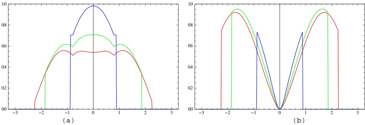
**FIGURE 4.** The simulations of the bifacial PV cell with the retroreflector (a) and the bifacial PV cell without the reflector plotted versus azimuth angle (rad.). Latitude:  $55.676^\circ$  North, Dates: (red) 23/6, (green) 10/4 and (blue) 21/12.
