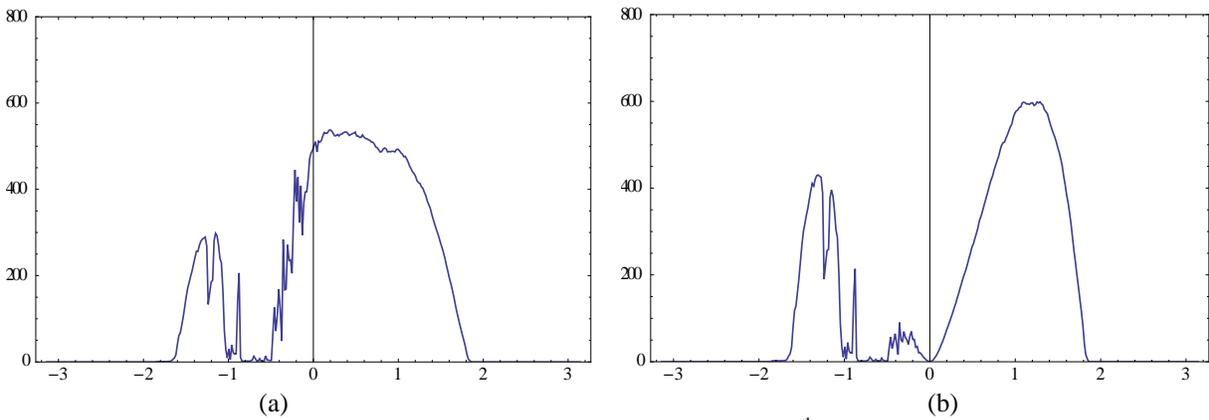
**FIGURE 6.** Simulations of solar power obtained near Copenhagen at the 10<sup>th</sup> April 2017 are plotted as a function of azimuth angle (rad.) for the prototype PV (a) and the reference PV (b).
