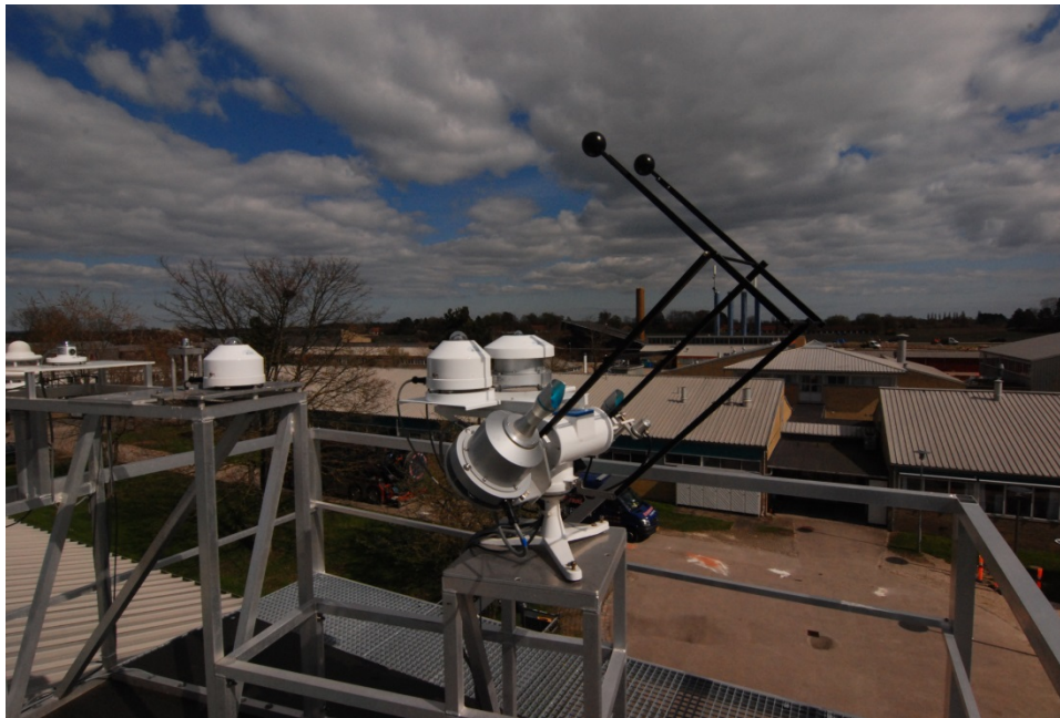
FIGURE 2. (a) The tracking solar setup and (b) the prototyping setup of the bifacial PV cell with its retroreflector are illustrated above.
