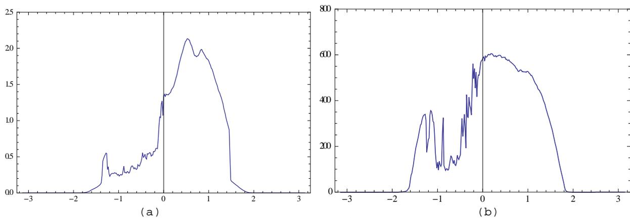
**FIGURE 7.** (a) Solar data obtained near Copenhagen at the 10<sup>th</sup> April 2017 by the prototyping bifacial PV cell with retroreflector is plotted as a function of azimuth angle (rad.) (b) The simulated irradiance including solar data for normal incidence and half the measured amount of diffuse light.
