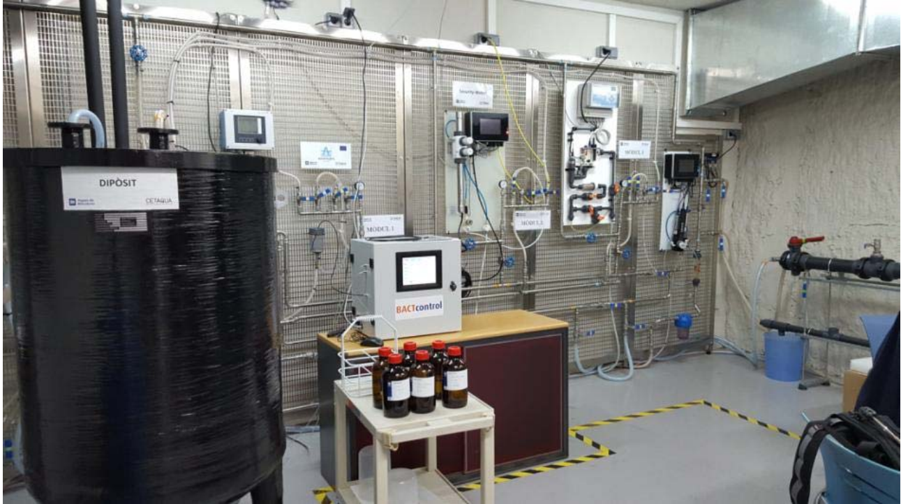
Figure 3. The BACTcontrol installed in a test rig at Aigües de Barcelona, the water supply for Barcelona, Spain.
