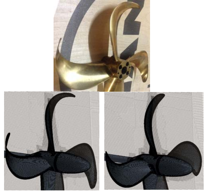
Figure 2: Experimental model (top) of tip-modified propeller and computational models of tip-modified (bottom left) and conventional (bottom right) propeller
