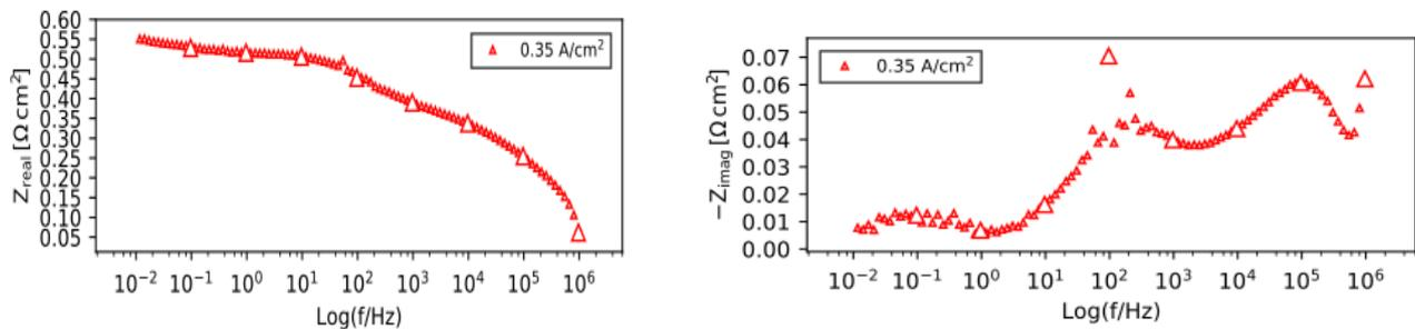
Figure 4. Real part (left) and Imaginary part (right) of the impedance of an EWII IrRuOx PEMEC as a function of log(frequency) at 61 °C and 0.35 A cm<sup>-2</sup>.
