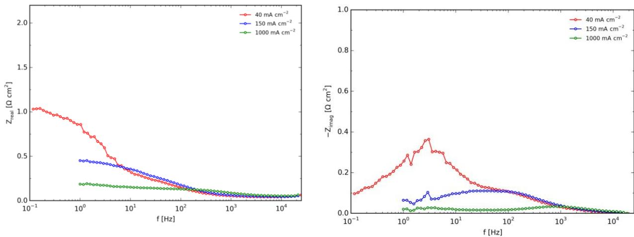
Figure 7. Real part (left) and Imaginary part (right) of the impedance of a Raney Ni AEC as a function of log(frequency) at 80 °C and 0.04, 0.15 and 1.00 A cm<sup>-2</sup>.
