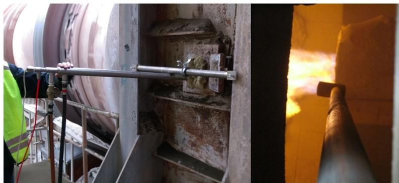
*Figure 1. Camera inserted through side of kiln hood next to burner.*
