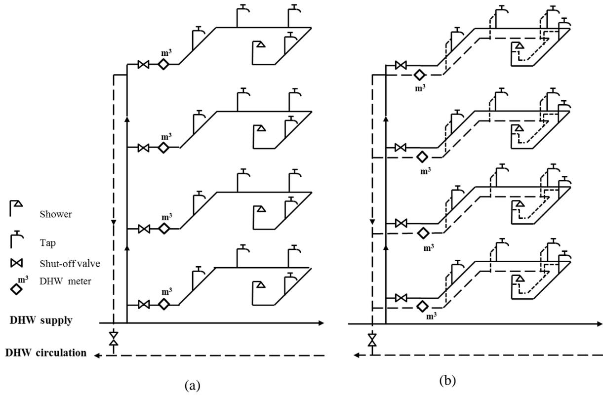
Figure 4. Two different circulation pipe arrangements
