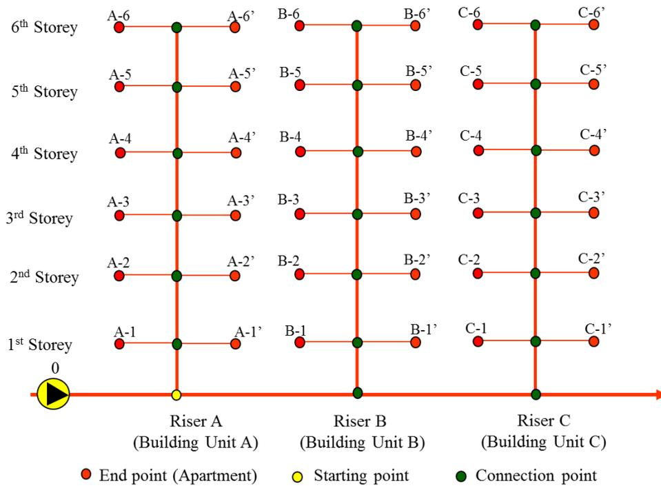
Figure 7. Graphic showing the heating installation structure
