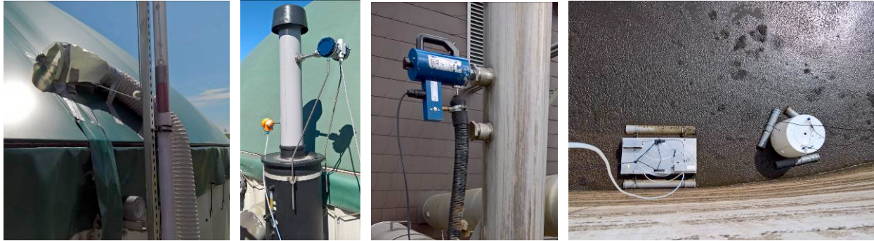
Figure 1. Single quantification methods of the on-site approach in field operation; from left to right: encapsulation and quantification of a leakage by means of an aerated windtunnel; permanent monitoring of pressure relief valves; right top: heated sampling at a conducted emission source (CHP off-gas); Chamber measurements at an open digestate storage tank with static and dynamic chambers (modified from Reinelt 2017).
