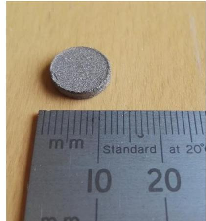
Figure 3: Sintered sample.
