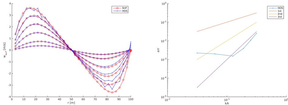
Figure 3: Left: Vertical velocity at free surface by cylindrical third-order HOS scheme, compared to stream function wave solution for varying  $kA$ . Right: Convergence of solution for vertical velocity for varying wave steepness  $kA$ .
