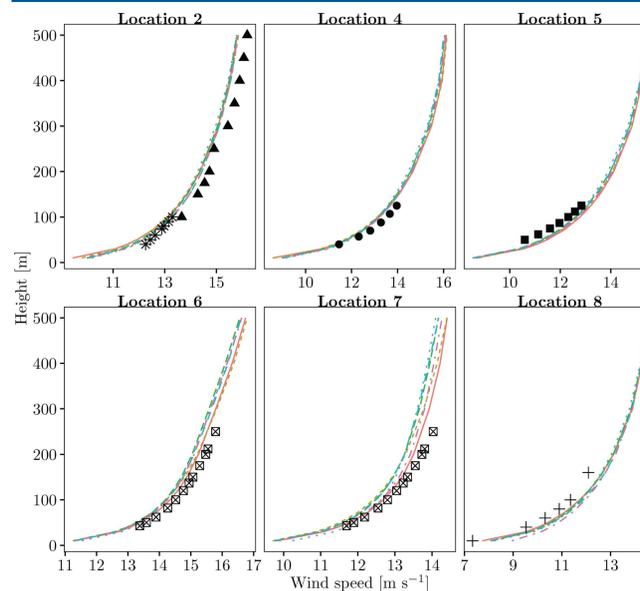
Mean vertical wind speed profiles at 6 different locations (see map at the left) observed by lidars and modelled with the MYJ scheme (abbreviations explained to the left).
