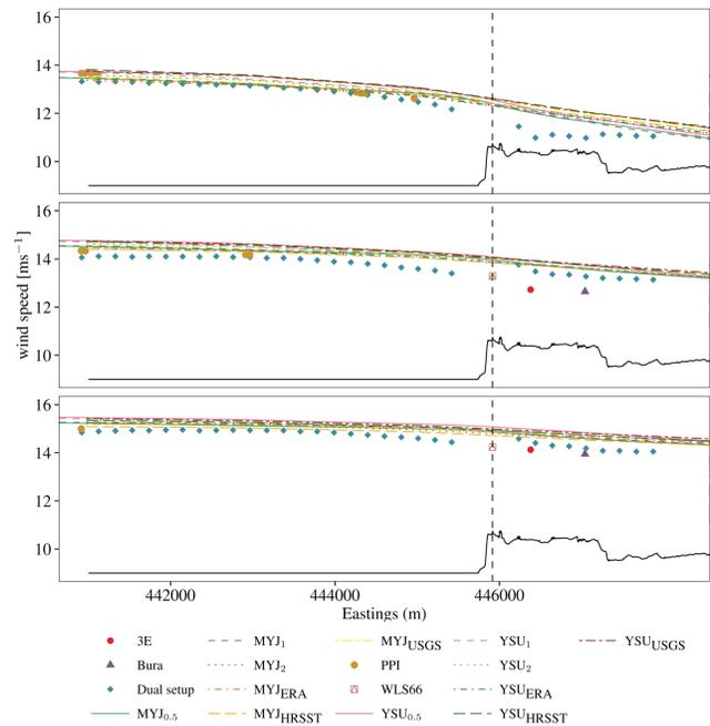
Generally the model prediction show slightly higher wind speeds offshore. Over land at 50 m the observed wind speed is much lower than the modelled wind. The WRF model cannot capture the effect of the cliff well, partly due to its coarser resolution.
