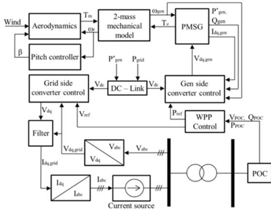
Fig. 2 Block diagram of the phasor model
