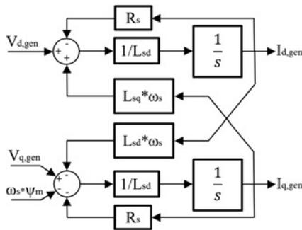
Fig. 7 Block diagram of the generator model
