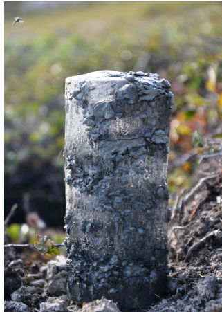
Figure 2.5: Large ice content is revealed in this back-lit photo of a 26 cm-long permafrost core from depth between 1.19 - 1.45 m. The core sample comes from a borehole drilled just 5 meters east of the automated ERT profile. ( photo: L. Pedersen )
