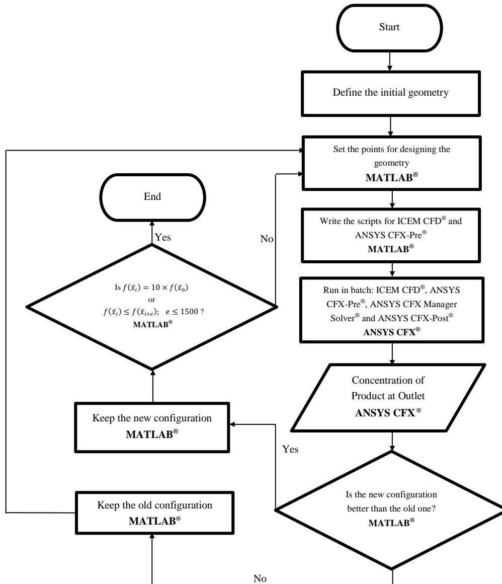
Figure 1 – Algorithm for the shape optimization of the enzymatic microreactor.
