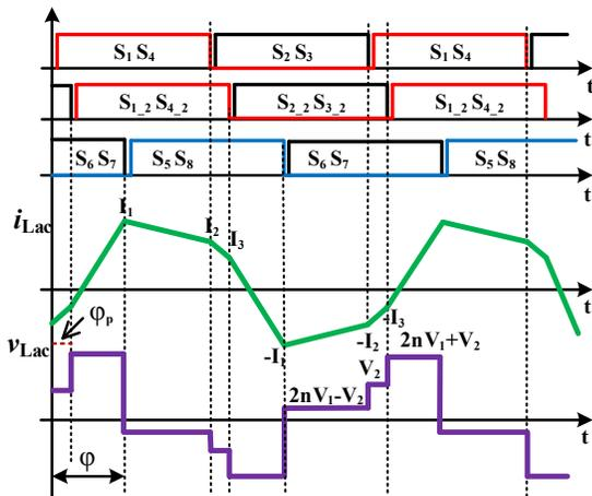
Fig. 3. Phase-shift control of the paralleled active bridges.
