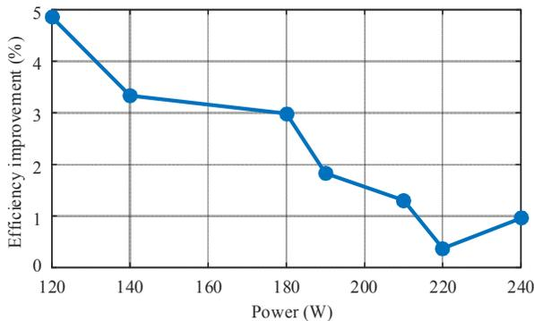
Fig. 10. Measured efficiency improvement at low power.
