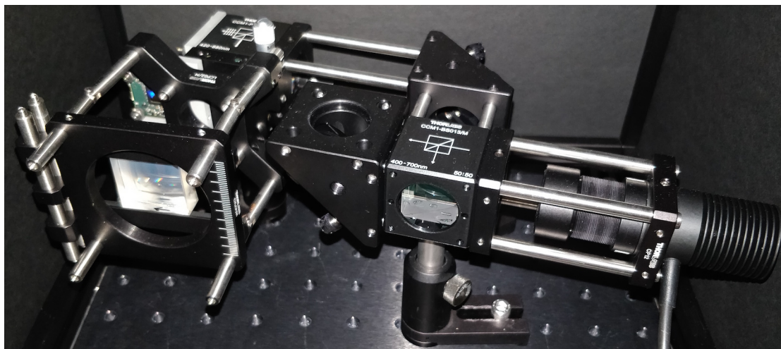
Figure 8.2. Photograph of compact setup, employing an LED light source and two CMOS cameras acting as a microscope and spectrometer, respectively. Microscope objective not shown.
