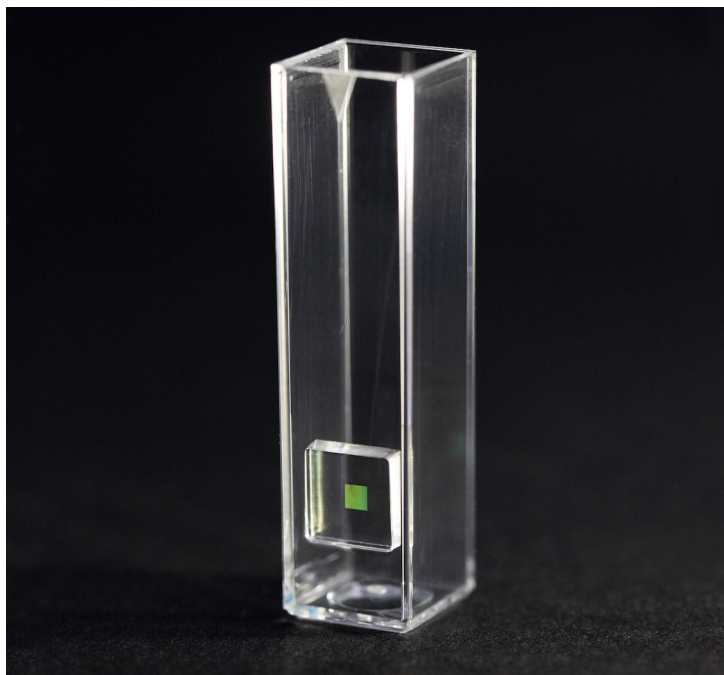
Figure 8.4. Photograph of early sensor-embedded cuvette. The presence of a PCS sensor allows a standard spectrophotometer to measure unperturbed absorbance in one orientation, and refractive index in the other orientation.
