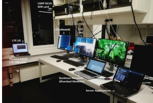
Fig. 6. The proposed co-simulation evaluation testbed.
