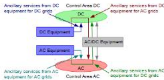
Figure 90: Overview of the four ancillary services in a power system in a single control area and with an both AC and DC grid (the grey arrows are responsibility-dependent and thus belong to AC or DC equipment).
