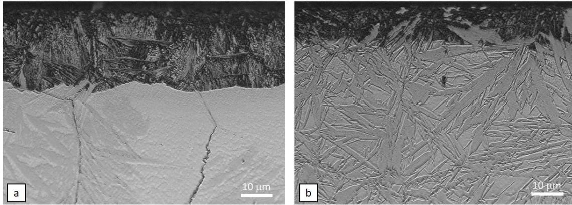
Figure 4: Reflected light micrographs showing the microstructure of samples HTSN+LTSH and HTSN+CRYO+LTSH. Etching with Murakami and HCl-modified Nital.
