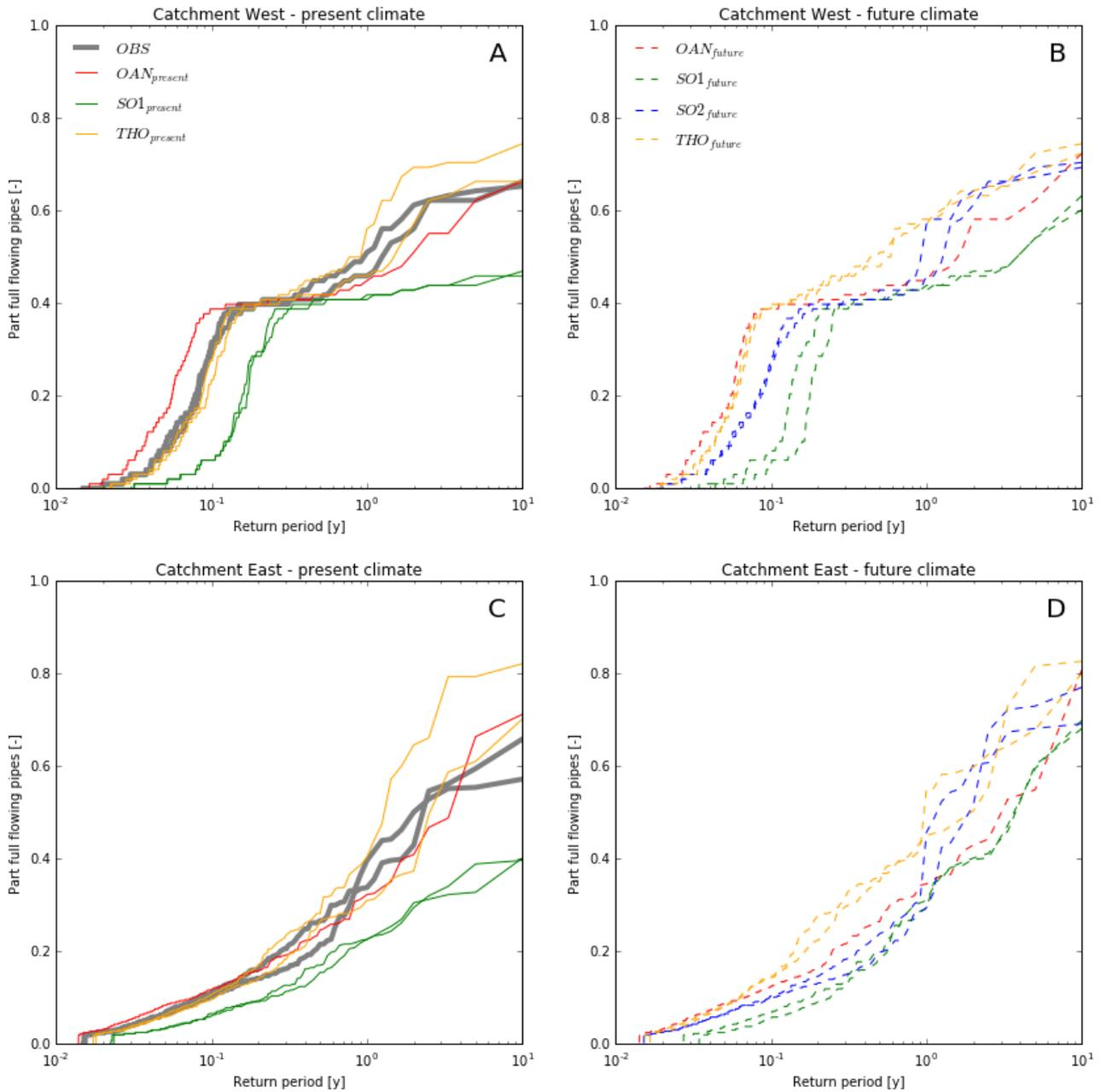
Figure 4 Part full flowing pipes for the different data sets for the Western (A+B) and the Eastern (C+D) catchments. *OBS* represents the same historically observed rainfall in all plots. For present climate *SO2* is by definition identical to *OBS*.
