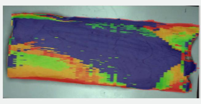
The augmented reality information of the fat layer thickness is shown to the operator as a colored fat contour in the HMI display and will guide the operator in where the belly should be trimmed. In a previous experiment a yield improvement in the order of 7-10% was demonstrated.
