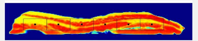
Digital Volume Correlation (DVC) is used in order to get the deformation field (mapping) between the belly geometry in the curved and flat state. This is used for adjustment and verification of the numerical finite element simulations. The two figures above show initial results in terms of mapping of a 2D cross-section of a belly including the contours indicating the Hounsfield scale, which is used to distinguish the different soft tissue constituents.
