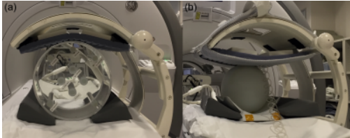
Figure 1: Coil setup for (a) the thermally polarized phantom experiment, and (b) the hyperpolarized phantom experiment. The pictures show the clamshell coil and the top paddle of the 16-channel receive array. The bottom paddle is under the linen. The phantom in (a) is a 20-cm long cylinder with 24 cm inner diameter and eight cylindrical compartments. Six of these are filled with 1.5 M [1-^{13}\text{C}] -L-Alanine, 2.0 M ^{13}\text{C} -Urea, and 2.0 M Sodium [1-^{13}\text{C}] Acetate, respectively, the last two are empty. The large compartment contains natural abundance Ethylene Glycol. The phantom in (b) is a sphere with 18 cm diameter.
