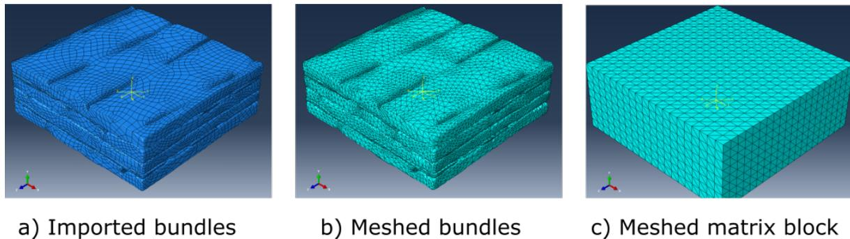
**Figure 5.** Example of workflow in ABAQUS
