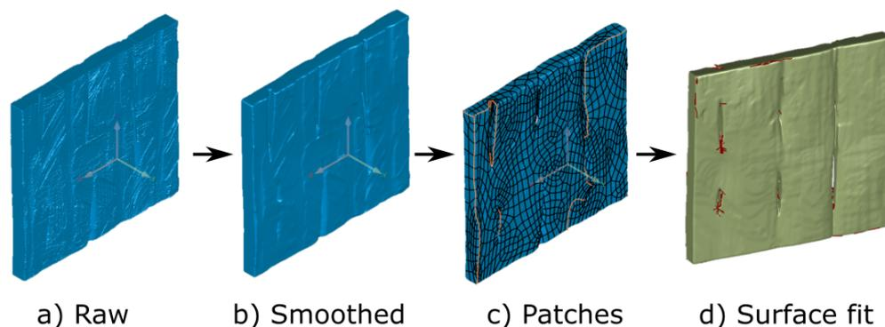
**Figure 4.** Example of workflow in Geomagic Wrap
