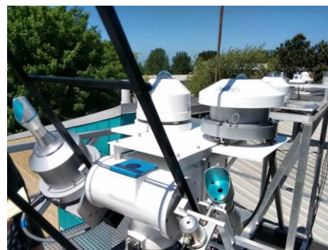
Fig. 1. The solar resource monitoring station at DTU Fotonik with instruments for measuring broadband and spectral solar irradiance.
