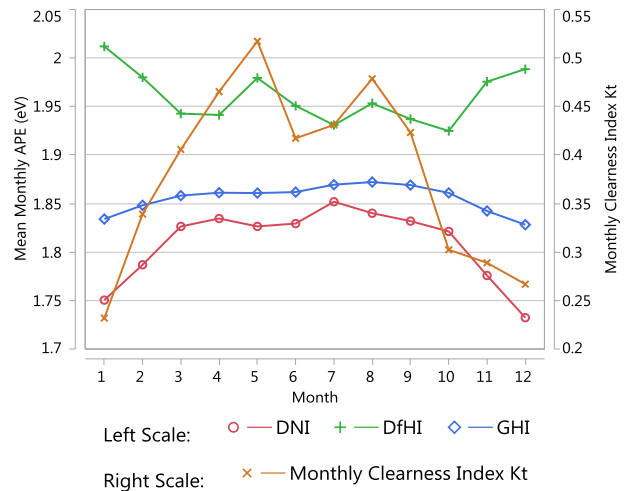
Fig. 6. Overlay of the mean monthly APE for the direct, diffuse and global irradiance components (left scale). The monthly clearness index ( K_T ) (right scale).
