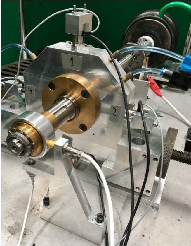
Figure 1.3: Picture of an experimental test rig consisting of a shaft with a disc attached to the end and a position controlled by an active gas bearing.
