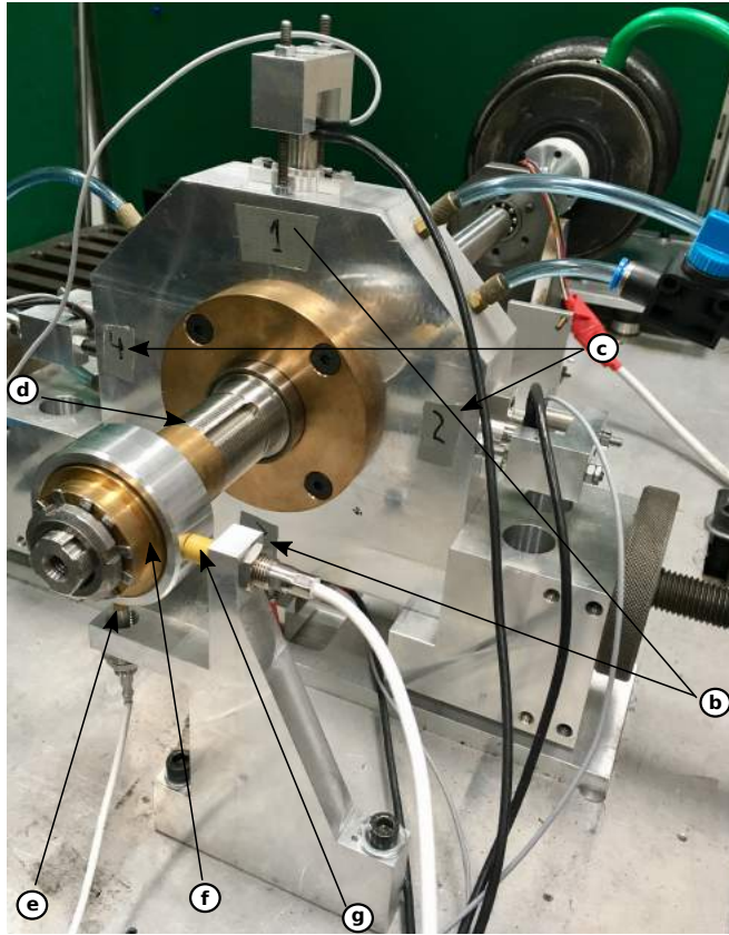
Figure 3.1: Picture of the experimental test rig, used for experimental validation of the methods introduced. The different parts of the test rig is as follows: b are the piezo actuators pumping air into the controllable gas bearing in the vertical direction, c are the piezo actuators pumping air into the controllable gas bearing in the horizontal direction, d is the flexible shaft, e is the sensor measuring the vertical displacement of the disc, f is the disc and g is the sensor measuring the horizontal displacement of the disc.
