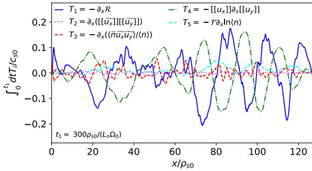
**Figure 2.** The radial profile of the terms of the right hand side of equation (9) for  $\alpha = 0.0005$  and  $L_n = 32 \rho_{s0}$ . The ZF signature of the radial advection term  $T_4$  is comparable to the Reynolds stress  $T_1$ .
