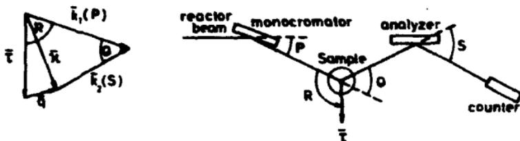
Fig. 4. Schematic diagram of the triple-axis-spectrometer.
