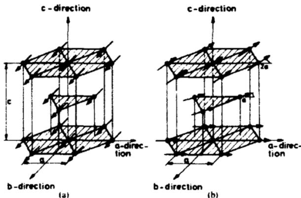
Fig. 1. The magnetic structure in terbium
