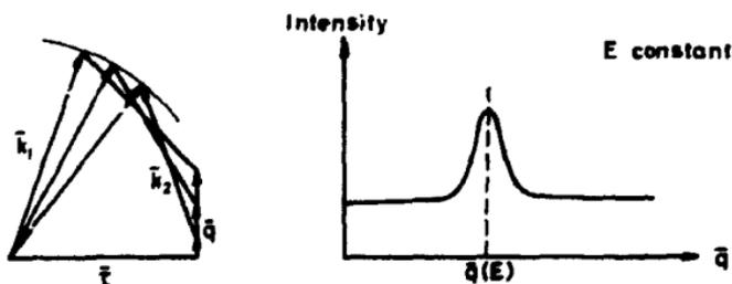
Fig. 5. Diagram illustrating a constant  $E$  scan.
