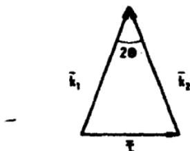
Fig. 2. Vector diagram for Bragg scattering.
