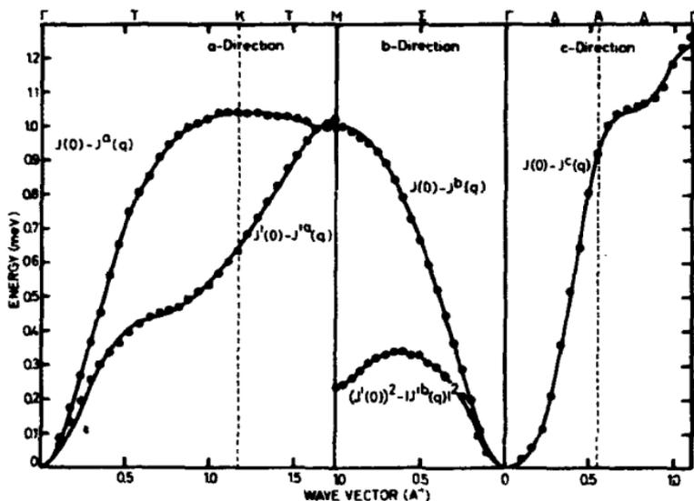
Fig. 23. Fourier transformed exchange parameters for Tb at 90 K.
