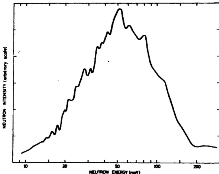
Fig. 16. Intensity of first order neutrons from the monochromator, as a function of neutron energy measured with the use of a quartz filter<sup>14</sup>. The spikes are due to parasitic reflections in the monochromator crystal.
