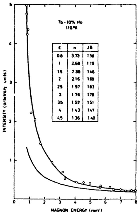
Fig. 21 Determination of the two-fold anisotropy parameter from the intensities of the inelastically scattered neutron groups.  $n$  is the ratio of the observed integrated intensity (the upper curve) and  $n_z(q) - 1$  (the lower curve) calculated from (25).
