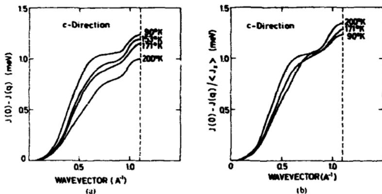
Fig. 26. (a) Temperature dependence of the Fourier transformed exchange parameters in the c-direction in the ferromagnetic phase of Tb.
