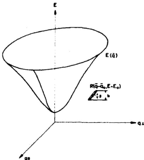
Fig. 14. Dispersion surface and resolution ellipsoid for  $\mathbf{q}$ -vectors in the scattering plane. In constant  $\mathbf{q}$ -scans the resolution ellipsoid is moved vertically through the dispersion surface.
