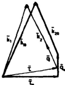
Fig. 9. Vector diagram showing how the finite collimations and mosaic spreads introduce an uncertainty in the  $\mathbf{q}$ -vector, because deviations of all vectors from their averages (labelled with subscript 0) are possible
