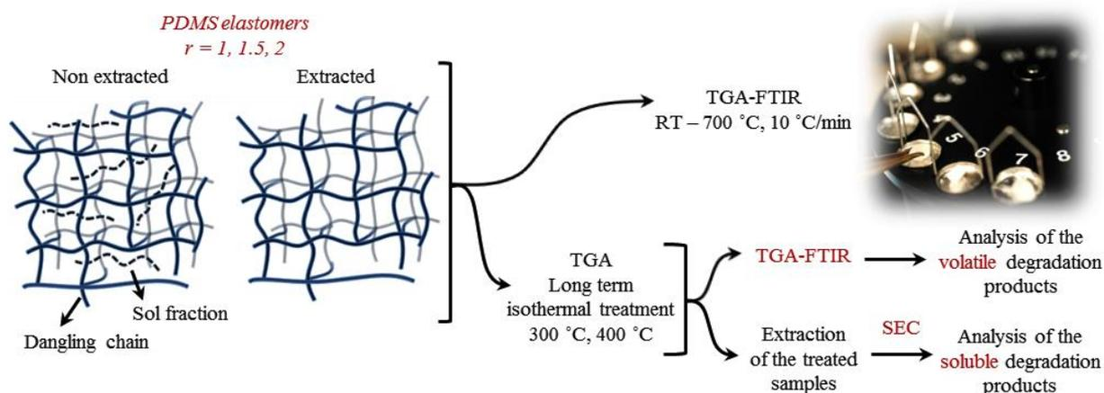
**Figure 1.** Scheme of the experimental procedure designed to investigate the thermal degradation behaviour of the silicone elastomers before and after removal of the sol fraction by extraction.
