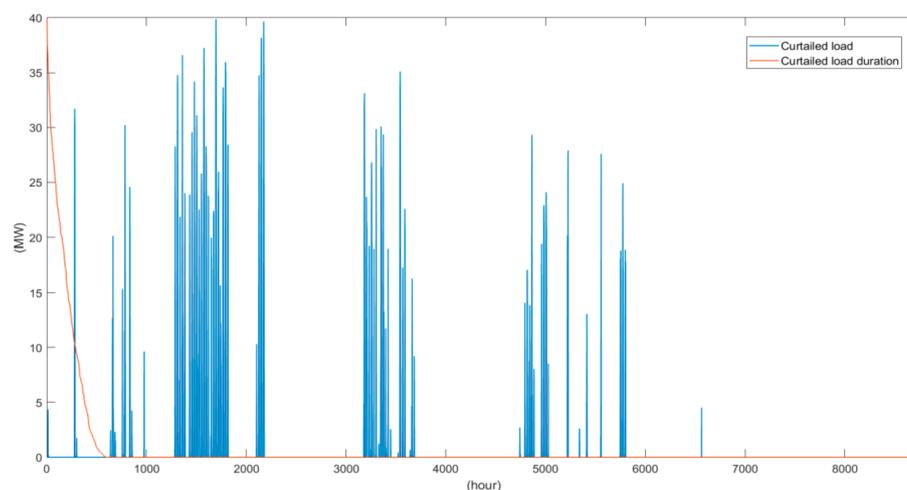
**Figure 2.** Curtailed energy in the energy system of 2020.
