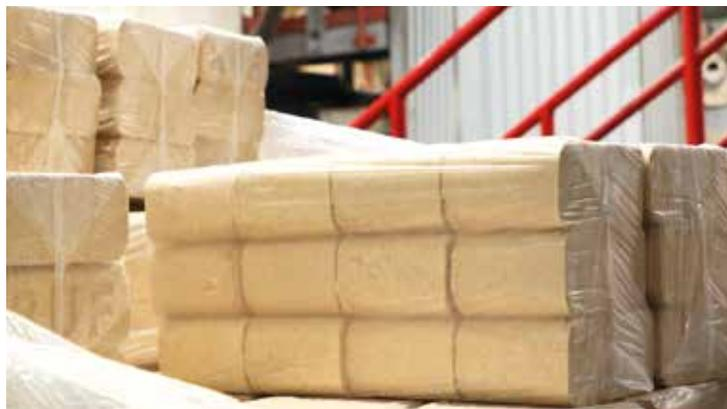
Wood briquettes have several advantages; they can be produced easily, flexibly and inexpensively with modern machinery precisely where wood residues occur. However, a disadvantage is that small-scale biomass boilers typically used in residential and light commercial space applications cannot be fed continuously and automatically with briquettes. This has a limiting effect on the potential local market for the producer.
