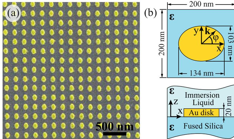
**Figure 1.** (a) False color SEM image of the fabricated anisotropic metasurface. (b) The structure consists of 20-nm-thick gold nanodisks arranged in a square lattice (period 200 nm). The base of the disks has an elliptical shape, with the long and short axes equal to 134 and 103 nm, respectively. We assume the environment is uniform and isotropic with  $\varepsilon = 2.1$ .
