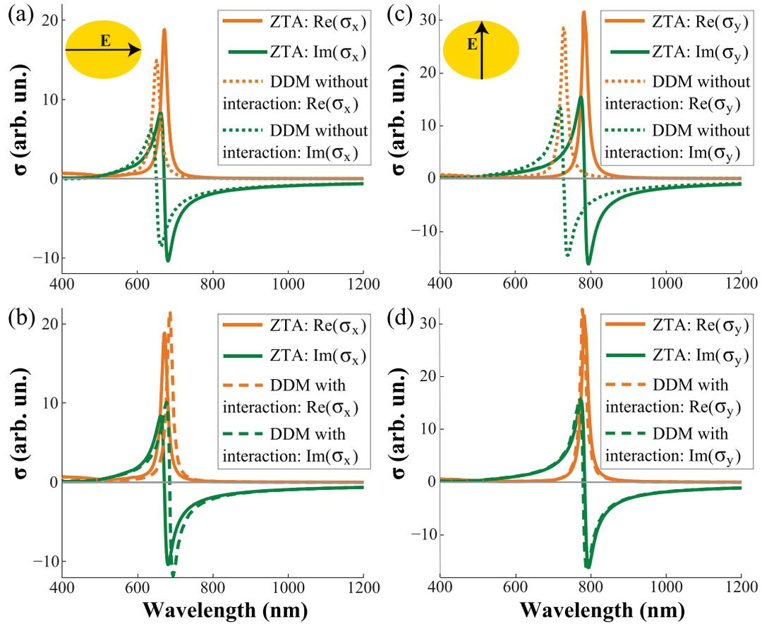
**Figure 3.** Real (orange lines) and imaginary (green lines) parts of the effective conductivity extracted via ZTA (solid lines), DDM without interaction (dotted lines) and DDM with interaction (dashed lines) for TM (a,b) and TE (c,d) polarizations.
