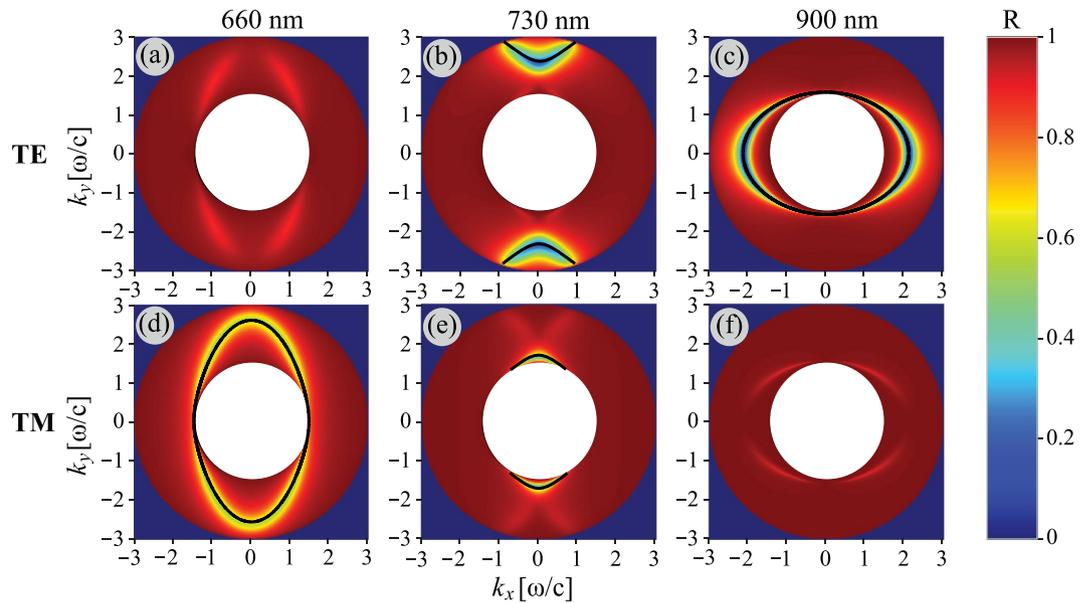
**Figure 5.** Simulation of the reflectance spectra from a metasurface shown in Fig. 1 for incident TE (a–c) and TM (d–f) polarizations. Panels (a) and (d), (b) and (e), (c) and (f) correspond to wavelengths  $\lambda = 660$ , 730, 900 nm, respectively. Black lines correspond to the equal frequency contours calculated from Eq. (6) straightforwardly. White circles correspond to the light cone with  $n = 1.45$ , while big circles correspond to the light line in ZnSe with  $n = 2.48$ .
