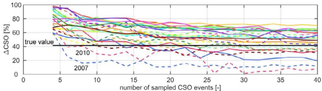
**Figure 4.** Estimated yearly reduction in CSO volume for the Lynetten example by using the simple sum of CSO volumes (dashed line) and the extrapolation method (solid line) as function of analysed events. Different years are visualized by using different colours. Lines shows the median value for the 100 realizations.
