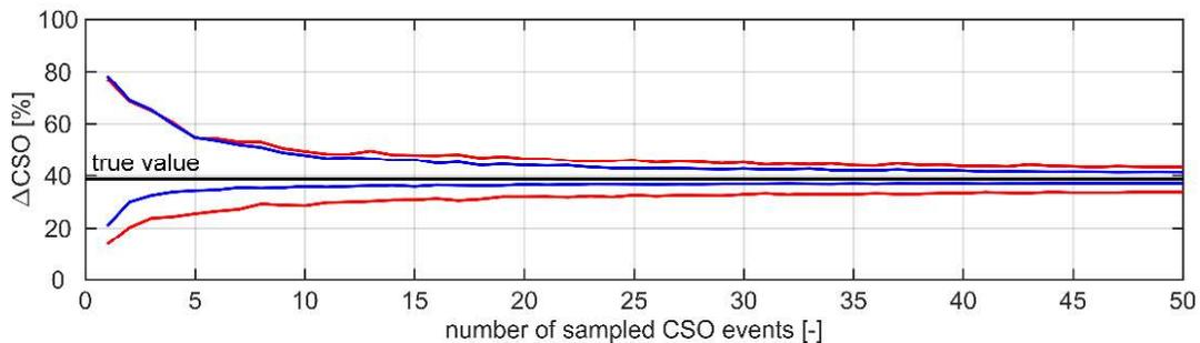
**Figure 3.** Estimated yearly reduction in CSO volume for the synthetic example by using the simple sum of CSO volumes (red) and the extrapolation method (blue) as function of number of sampled events. The lines show the 5-95 percentiles for the 100 realizations.
