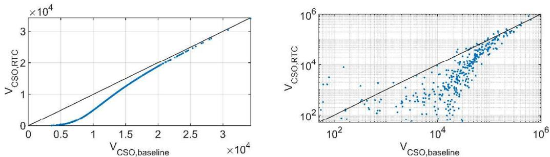
**Figure 2.** Comparison between CSO volumes without control (x-axis) and with control (y-axis) for all the analysed events. (left) Synthetic example. (right) Results for an integrated MPC strategy in the Lynetten catchment.
