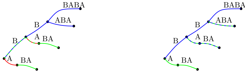
(a) The suffix tree of the string BBBABA , colored corresponding to attractor positions 2, 5, 6 . This attractor is minimal: removing any position leaves some edge uncolored.
