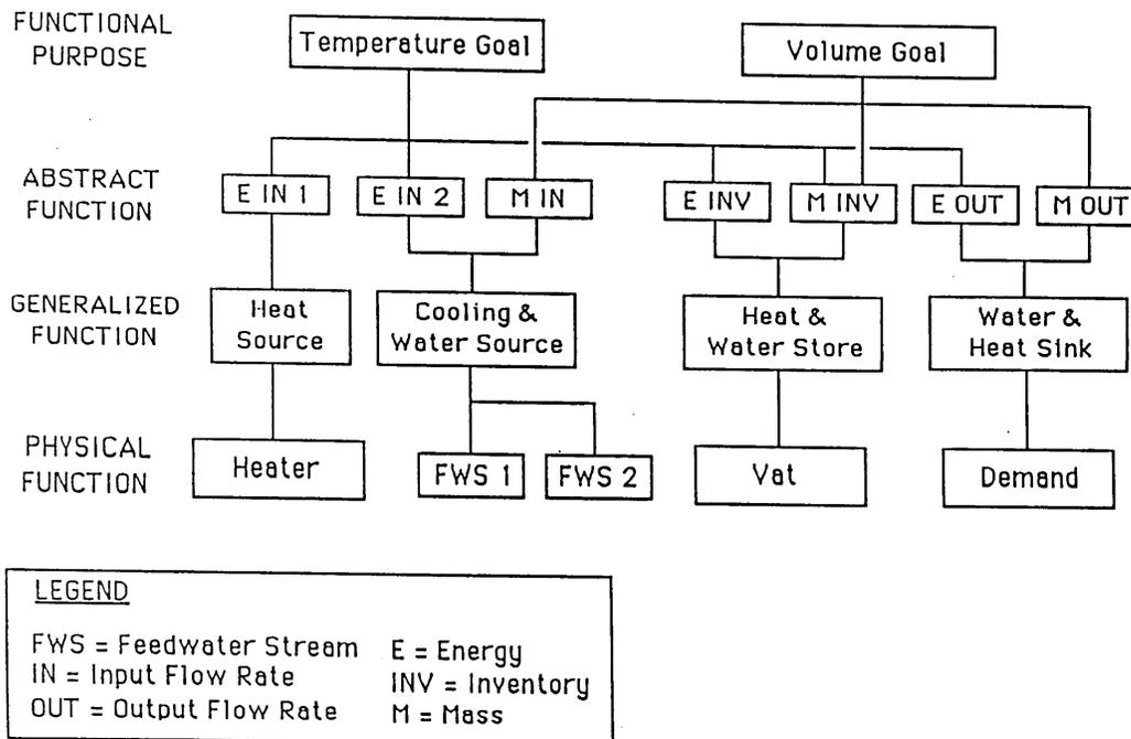
Figure 7. The mappings between the levels of the means-end hierarchy for DURESS.
