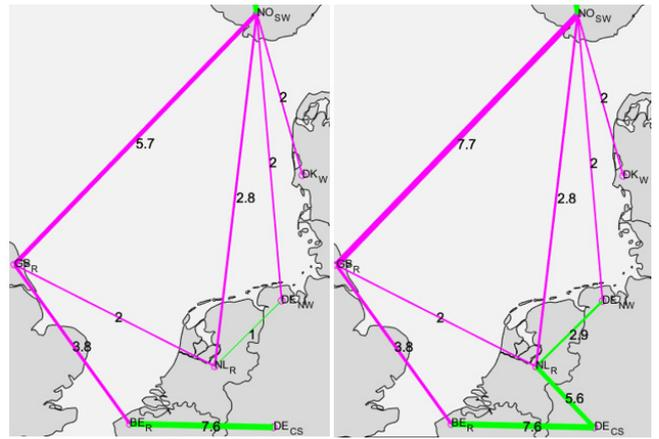
Figure 6. Endogenous transmission investments in 2030 on the left and accumulated investments by 2050 on the right for the radial scenario (GW). On-land lines are in green and offshore lines in magenta.
