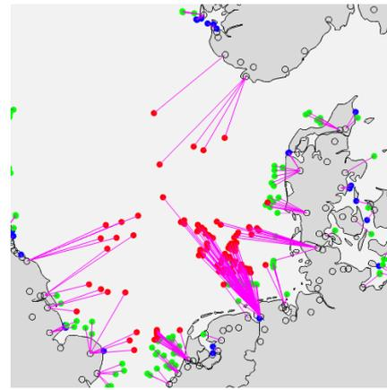
Figure 2. OWPPs used to estimate investable offshore wind capacities in the radial scenario: blue denotes nearshore, green HVAC connected offshore and red HVDC connected offshore OWPPs.
