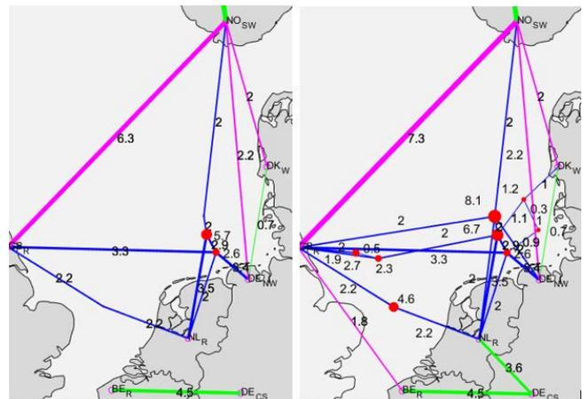
Figure 7. Endogenous transmission and hub investments in 2030 on the left and accumulated investments by 2050 on the right for the meshed scenario (GW). Radial offshore lines are in magenta, lines related to the meshed grid in blue, on-land lines in green, and hubs in red.
