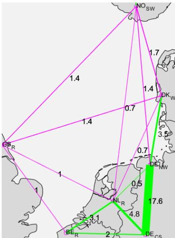
Figure 5. Assumed exogenous transmission development in the North Sea region (GW). Capacities, not actual locations of the lines, are illustrated. On-land lines are in green and offshore HVDC lines in magenta ( $DK_w$  to  $DE_{NW}$  is on-land, even though it appears offshore in the figure).
