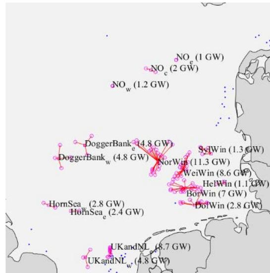
Figure 3. Investable hub-connected offshore wind capacities in the meshed scenario. The OWPPs connected to UKandNL<sub>w</sub> are British, and the ones connected to UKandNL<sub>e</sub> are Dutch. DoggerBank and HornSea consist of British OWPPs, and all hubs ending in “Win” consist of German OWPPs.
