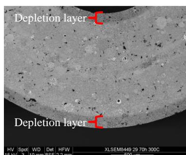
**Figure 1.** SEM image of catalyst pellet after 70 h on stream, at reaction conditions: temp. = 300 °C, feed = 4.4% MeOH, 10% O<sub>2</sub> in N<sub>2</sub>. Light gray indicates Mo rich composition (Mo/Fe = 2.6) and dark gray stoichiometric composition (Mo/Fe = 1.5).
