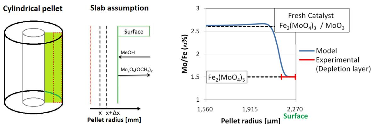
**Figure 2.** Left: Drawing of the catalyst pellet and 1D slab assumption model.
