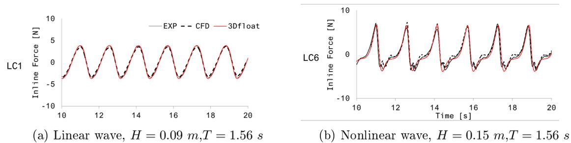
Figure 5: Comparison of computations with STAR-CCM (CFD), experiments from the WaveLoads project (Exp) and computations via the aeroelastic code 3DFloat. Reproduced from figure 15 in [14]
