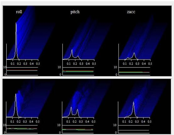
Figure 5 Transition of the auto-spectra of roll, pitch and vertical acceleration (zacc) (upper: min, lower: 1min).
