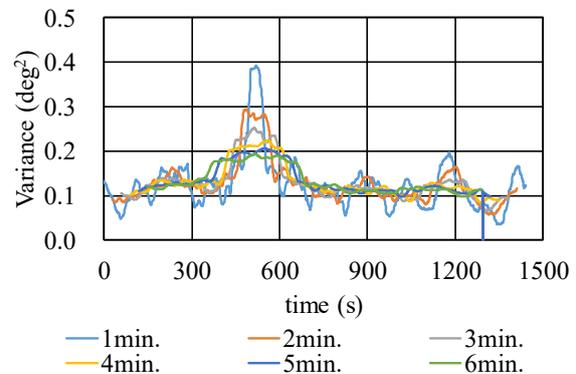
Figure 6 Transition of the pitching variance for each time spans (run C).
