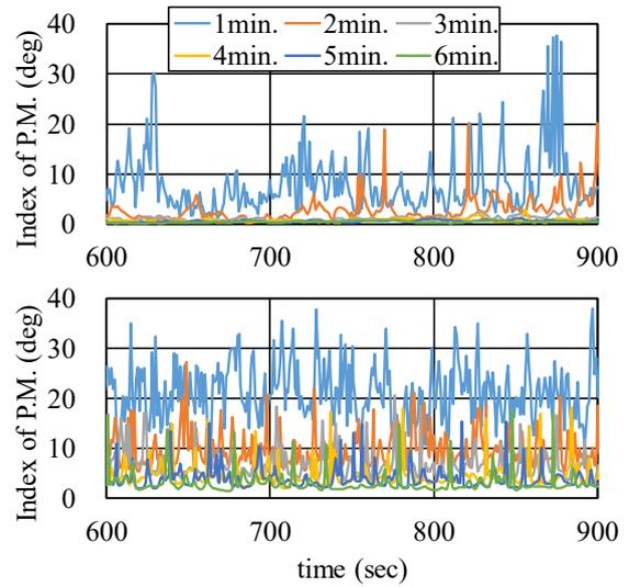
Figure 8 Transition of  $I_{PM}(n)$  of roll-pitch cross-spectra for each time span (runC).
