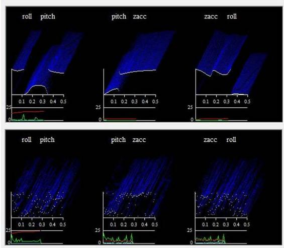
Figure 7 Transition of the relative phase angle between roll-pitch, pitch-zacc and zacc-roll. (upper: MAR, lower: DFT).
