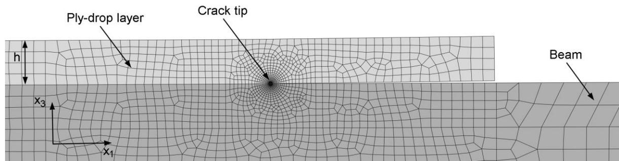
**Figure 9.** Plane strain finite element model to compute the mode I and mode II stress intensity factors for a delamination of a fixed length in ply-drop specimens of type A. (the deformed mesh is scaled to illustrate the crack opening).
