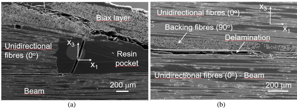
**Figure 6.** ESEM photographs of a ply-drop specimen of type B (Fig. 1c) after fatigue tests: a) View of the failure mechanisms at the first ply-drop, b) detailed view of the crack path between the ply-drop layer 1 and the composite beam.
