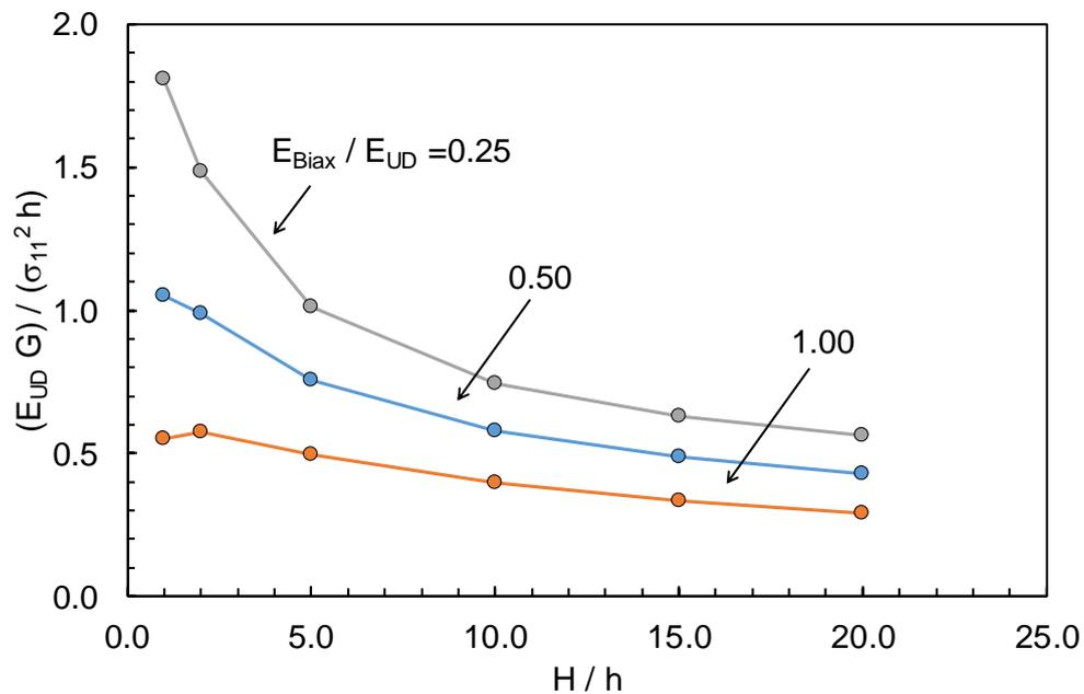
**Figure 8.** Effect of the beam height,  $H$ , and biax layer Young's modulus,  $E_{Biax}$ , on the steady-state energy release rate of the tunneling crack. The Young's modulus of the ply-drop layer and the beam is  $E_{UD}$  and the height of the ply-drop layer is  $h$ .
