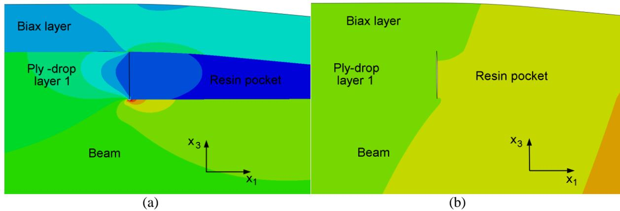
**Figure 7.** Plane strain finite element models to analyse the tunneling crack at the ply-drop layer / resin rich area interface: a) model to extract stresses at the interface (stress  $\sigma_{11}$  contour), b) mode to extract crack openings (displacement  $u_1$  contour).
