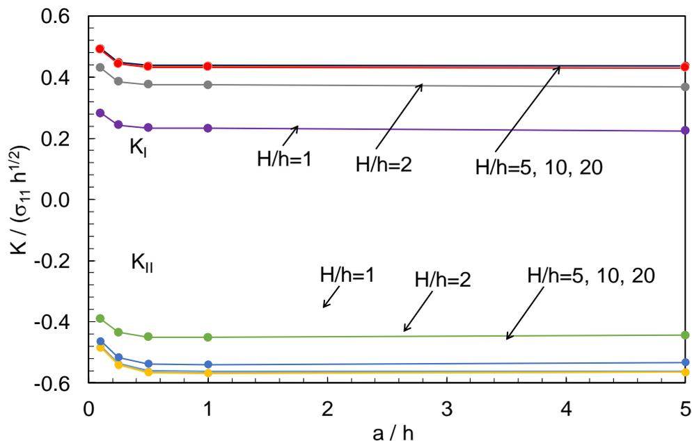
**Figure 10.** Mode I and mode II stress intensity factors as a function of the delamination crack length for the ply-drop specimen of type A (Fig. 1b) for different beam to ply-drop layer thickness ratios.
