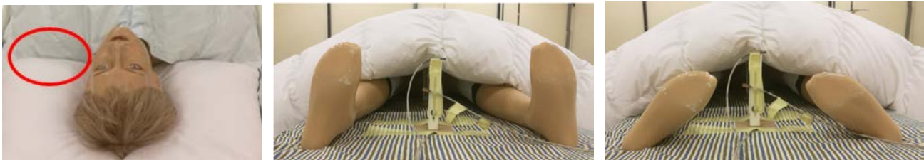
Figure 6. Sealed neckline – left; Position of feet: straight – middle; tilted – right.
