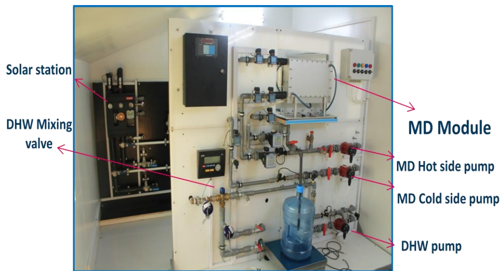
Figure 3: Solar Station and MD Circuit [28,30]
