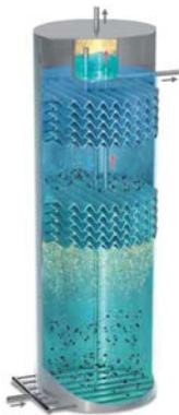
Water with high content of organic carbon dissolved enters at the bottom of the tank. In the bottom compartment, the anaerobic granular biomass converts organic compounds to  $\text{CH}_4$  and  $\text{CO}_2$ . In the upper compartment, biomass is retained by settling. (Picture: BIOPAQ®IC)
